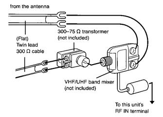
• If your television has both lead and coaxial VHF terminals, use the lead connection to minimize signal loss.
